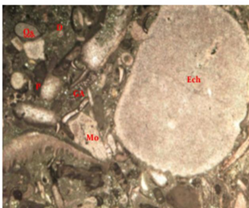
Plate.2. shows poorly sorted with Packstone texture. The main grain types are large echinoderm (Ech), Mollusca (Mo), Ostracoda (Os), peloids (P) and rare green algae (GA). Ground mass composed of very fine crystals of dolomite (D). Subtidal/Back shoal Dolomite/Limestone facies: Dolomitized Bioclastic Wackestone Microfacies.
