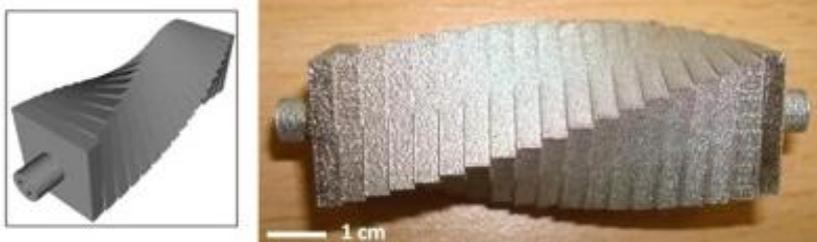
Figure 1: Showing poor surface finish
