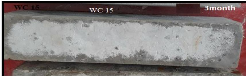
Figure 10. Geopolymer Mortar After 90 days of Exposure to MgSO<sub>4</sub> for WC.
