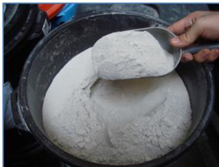
Figure 3: QD after grinding by LA Abrasion Machine
