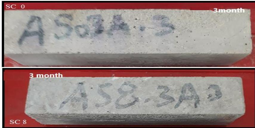
Figure 9. Geopolymer Mortar After 90 days of Exposure to MgSO<sub>4</sub> for SC and WC.
