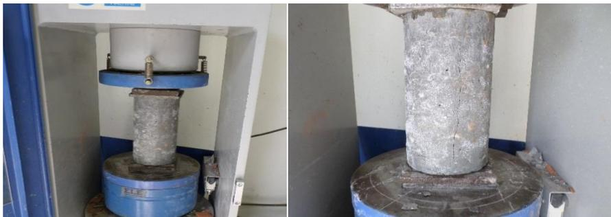
a) Compressive Strength Test      b) Crack propagation at failure due to compressive strength test
