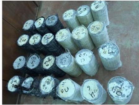
Figure 6. Specimens wrapped with CFRP/GFRP
