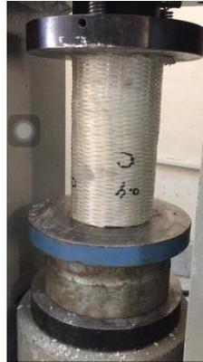
b) GFRP strengthened specimen
