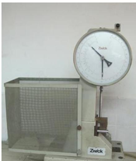
Figure 1. Zwick pendulum
