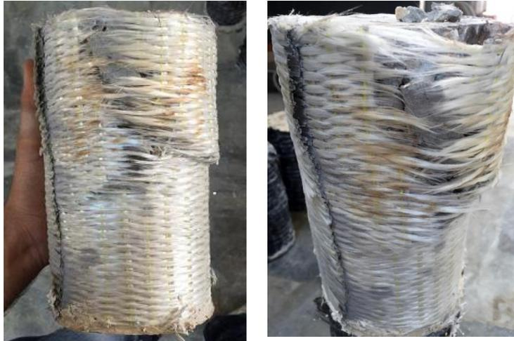
Figure 9. GFRP rupture
