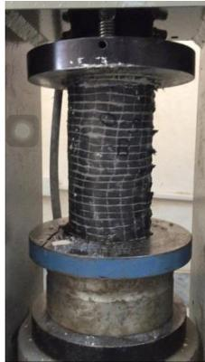
a) CFRP strengthened specimen
