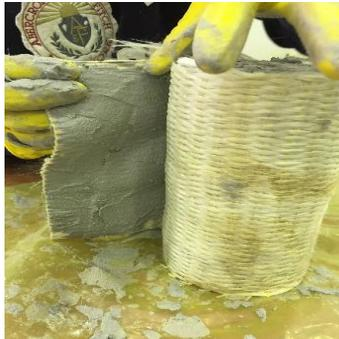
Figure 5. Glass Fiber wrapping for Cylindrical Column
