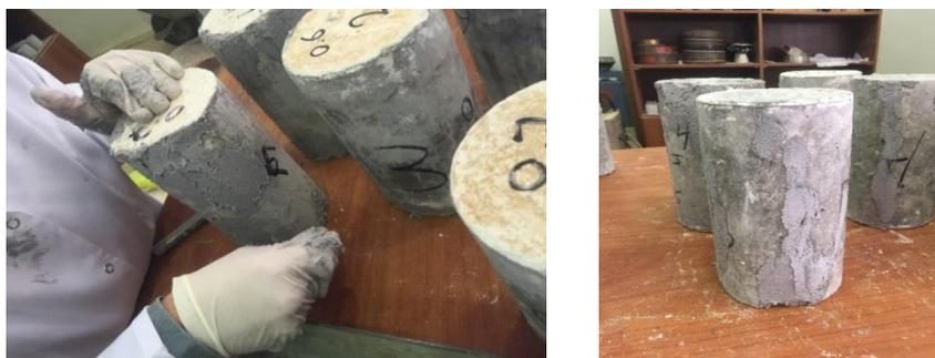
Figure 4. Cracks repair using an epoxy paste material
