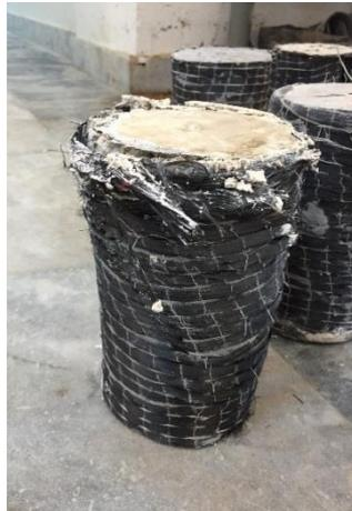
Figure 10. CFRP delamination failure
