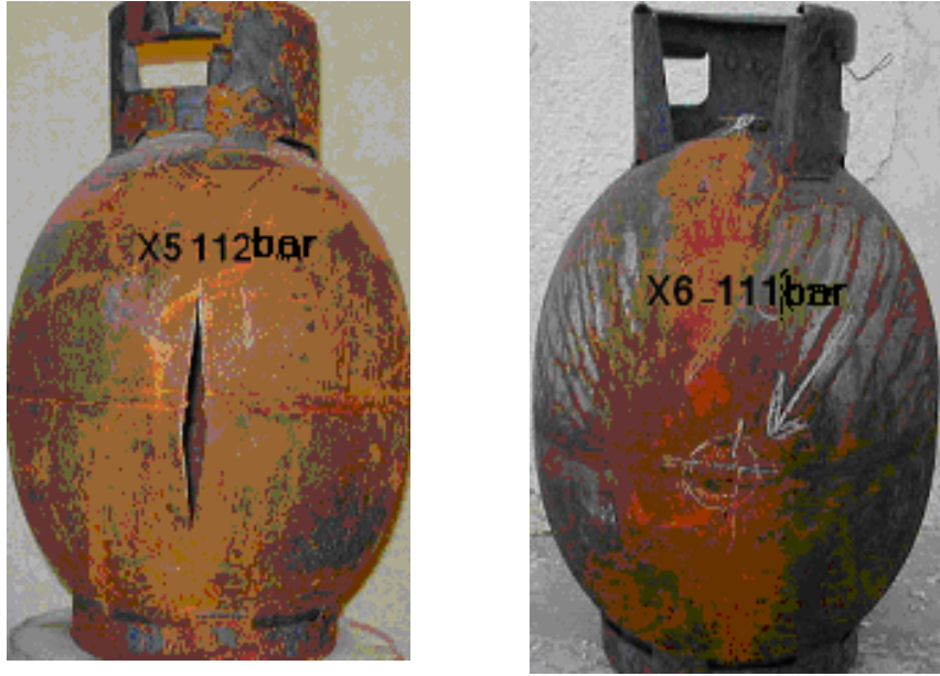
Figure (10) Burst shape of the (X) samples
